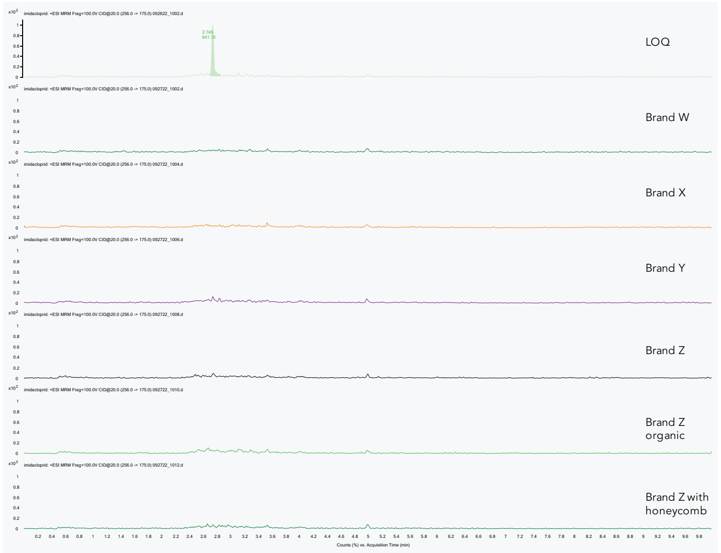
Figure 5: Representative stacked mass chromatograms for imidacloprid from an extracted LOQ honey standard (A) compared to extracted raw and unfiltered honey samples of Brand W (B), Brand X (C), Brand Y (D), Brand Z (E), Brand Z organic (F), and Brand Z with honeycomb (G).
