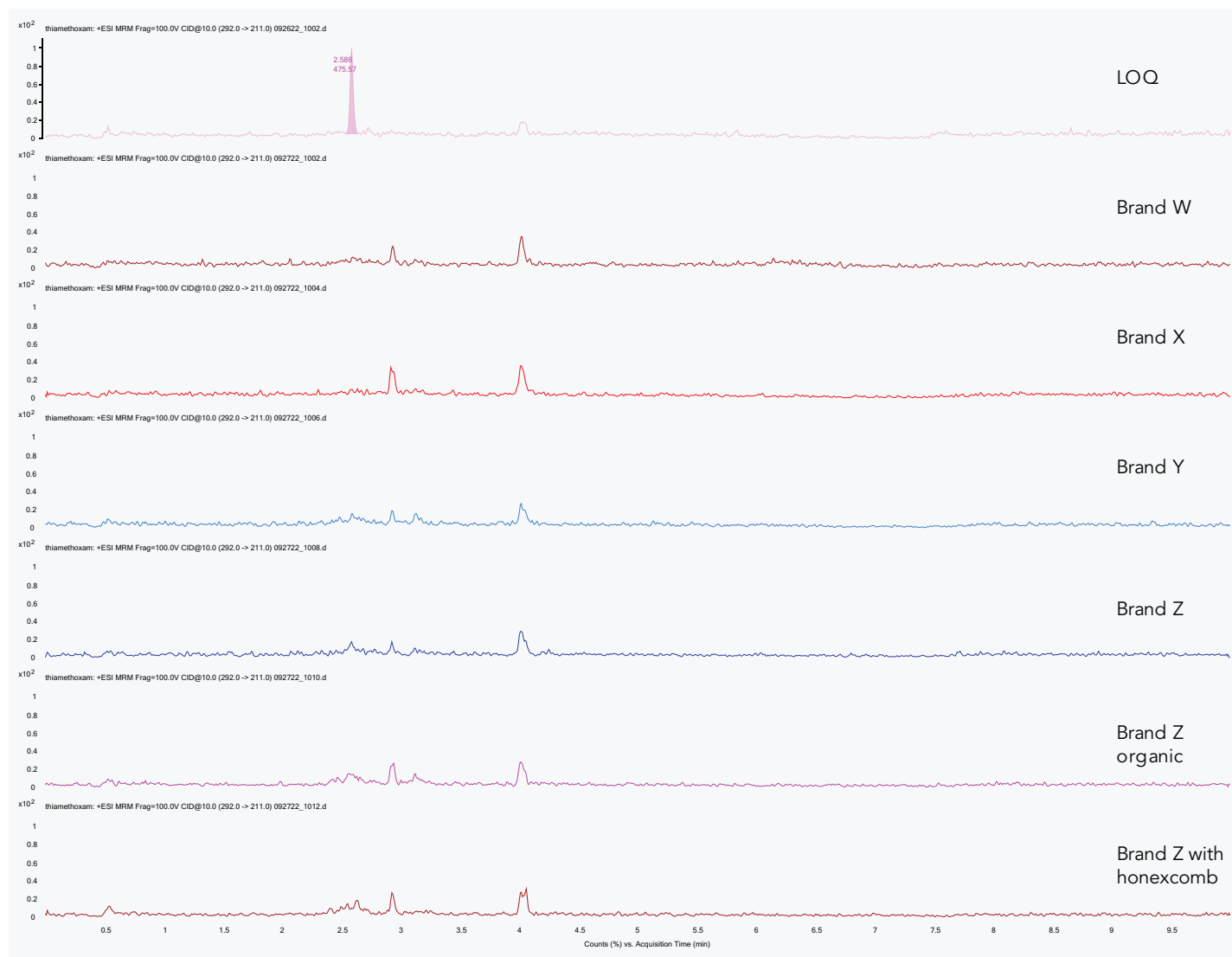
Figure 6: Representative stacked mass chromatograms for thiamethoxam from an extracted LOQ honey standard (A) compared to extracted raw and unfiltered honey samples of Brand W (B), Brand X (C), Brand Y (D), Brand Z (E), Brand Z organic (F), and Brand Z with honeycomb (G).
