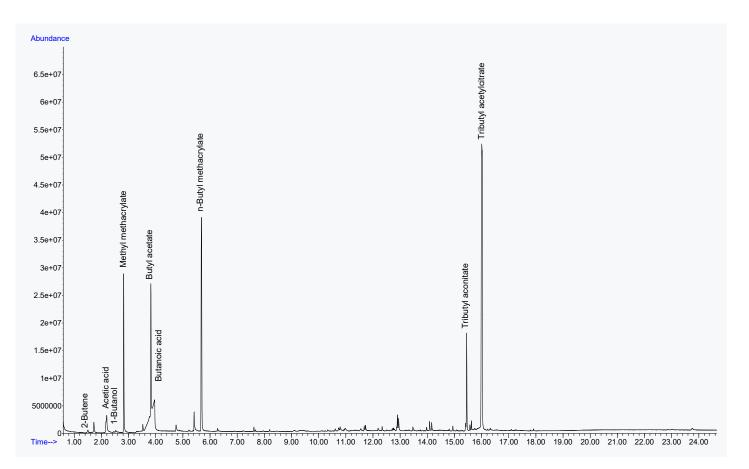
Figure 6: Pyrogram for acrylic nail hardener.
