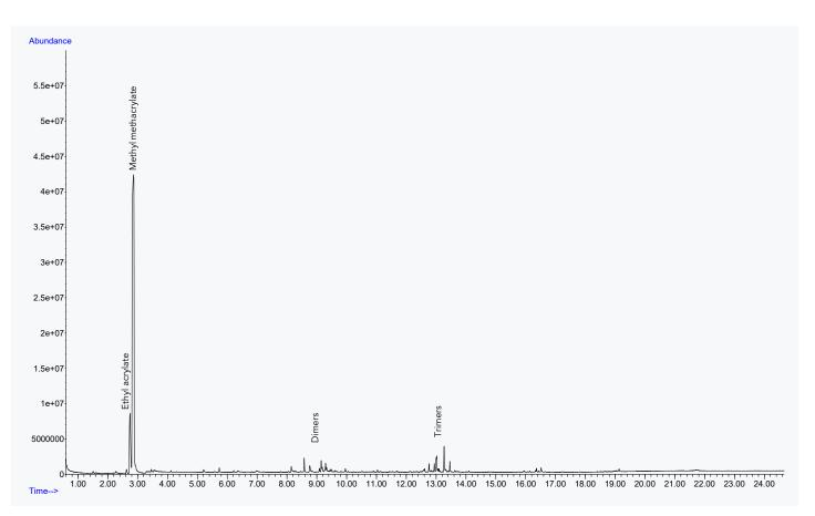
Figure 5: Pyrogram for plastic photo holder.
