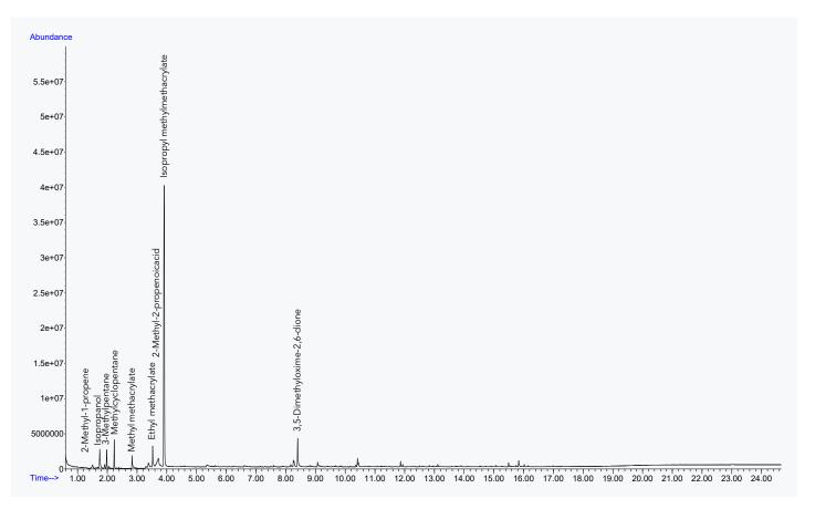
Figure 2: Pyrogram for polymethyl methacrylate.
