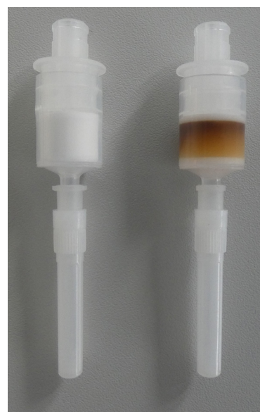
Figure 4: SPE cartridge before (left) and after (right) cleanup of a coffee extract.
