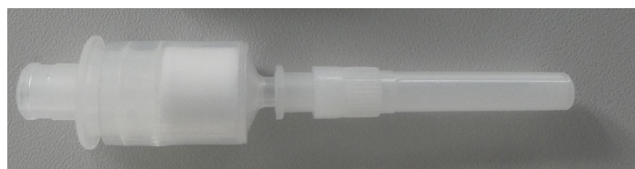
Figure 2: CHROMABOND® ABC18, 6 mL, 500 mg SPE cartridge (MACHEREY-NAGEL) equipped for automated handling with the GERSTEL MPS.
