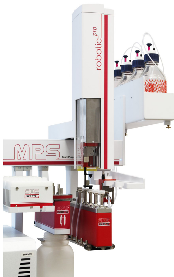
Figure 3: SPE module and cartridge tray mounted on a MultiPurpose Sampler (MPS). All solvents are delivered by an automatically exchangeable syringe in the autosampler head.
