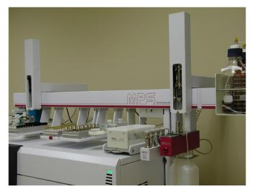
**Figure 2:** MultiPurpose Sampler (MPS XL) with GERSTEL SPE Option.
