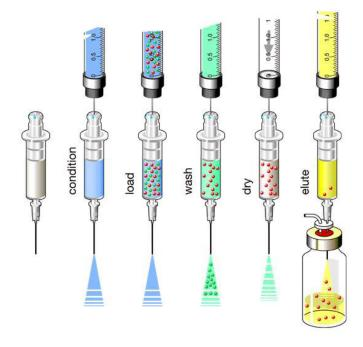
**Figure 1:** Graphical representation of a typical automated SPE procedure.
