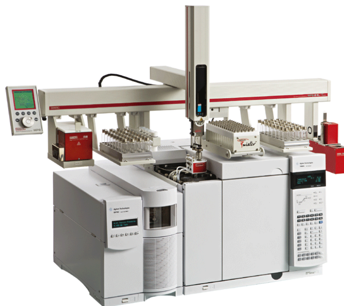
Figure 1: GERSTEL LabWorks Platform with DHS on an Agilent Technologies 7890 GC.
