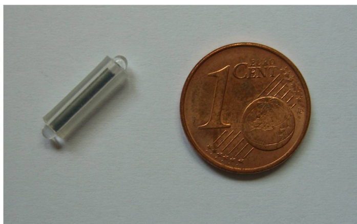
Figure 1: The GERSTEL Twister, used for stir bar sorptive extraction of drugs and pharmaceuticals from brain tissue in the work reported here.
