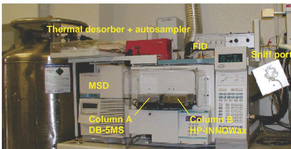
**Figure 1.** Multidimensional GC-GC instrument used for the study.
