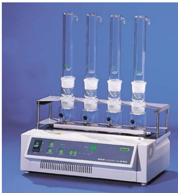
Figure 1. Büchi extraction unit B-815 for simultaneous extraction and saponification of fat according to the Caviezel method.
