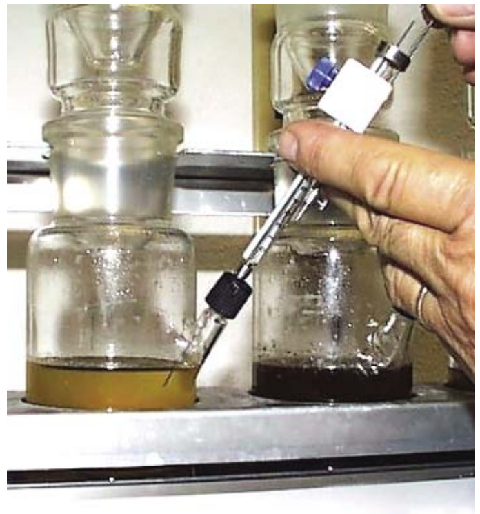
Figure 3. Taking a sample aliquot for GC analysis.
