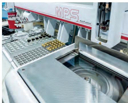
GERSTEL MultiPurpose Sampler (MPS) equipped with centrifuge, <sup>m</sup>VAP and QuickMix.
