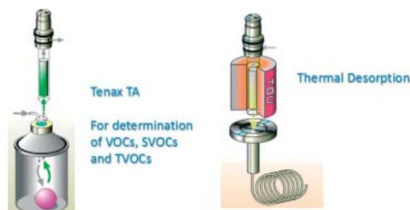
Figure 12. Tenax TA/TD-GC/MS method for the determination of VOCs, SVOCs and TVOC.
