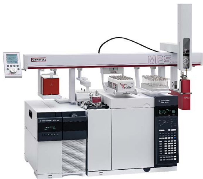
Figure 1. GERSTEL MPS-DHS-TDU Agilent 7890/5977 GC-MSD system.
